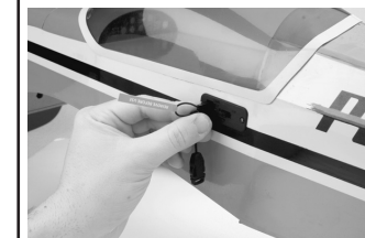
A, B. Insert bind plug into charge jack, apply power
